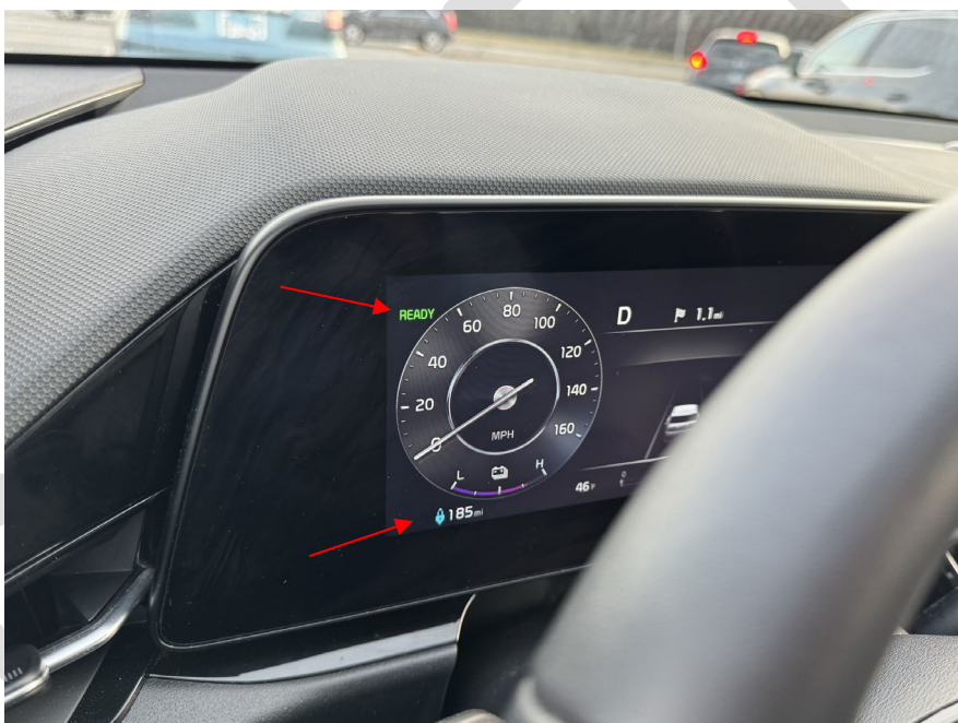
Figure 8 Instrument panel of a Kia Niro, as viewed from the driver's side doorway. Note the green "READY" indicating that the HV battery can supply power to the inverter/wheels, air conditioning, or other HV consumers.
