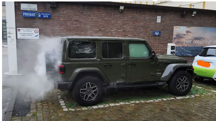
Figure 15 Example of a vehicle that has filled with battery vent gases – note the white smoke.
