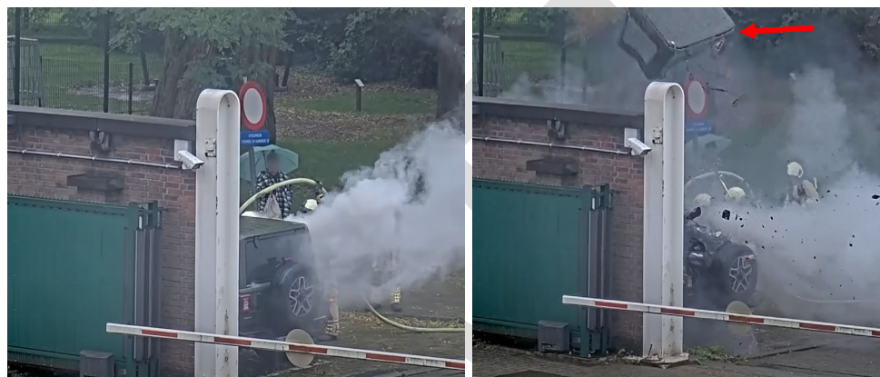
Figure 5 Screenshot of a video showing white fog emanating from a vehicle (left), followed by a screenshot after an explosion occurred where the roof of the cab has been pushed off of the vehicle (see red arrow). First-responders opened a window or door prior to the incident to ventilate the cabin. 33
